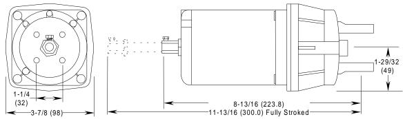
Figure 2: D-4073 Dimensions, inches (mm)
