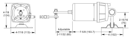
Figure 4: D-4073 with Auxiliary Mounting Bracket, inches (mm)
