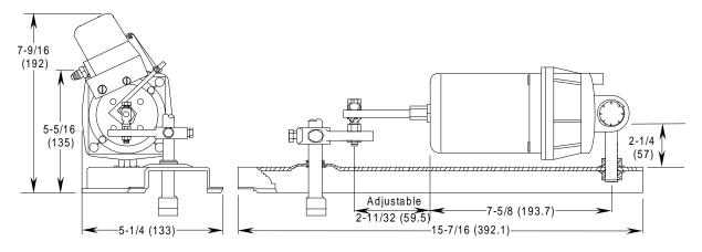
Figure 3: D-4073 with Universal Mounting Bracket and Pilot Positioner, inches (mm)
